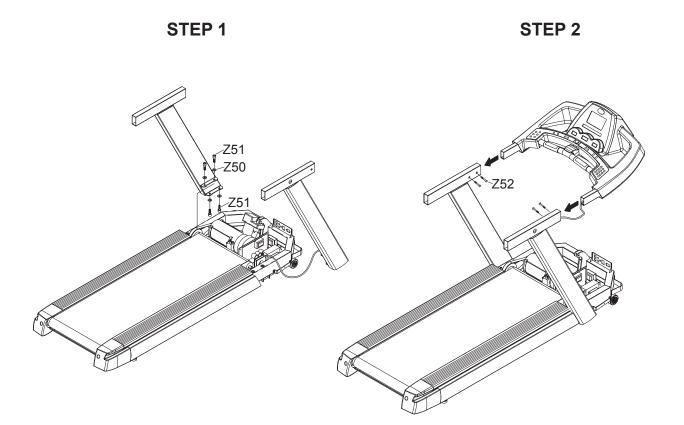
Remove the motor cover. Pull out the console cable and route it through the Right console mast. Place the right console mast and then the left console mast in the console post support brackets. Secure the Right and Left mast with the 4 bolts provided (Z50, Z51). Make sure these bolts are tight. Connect the console cables from the console set to the motor control board cables. Secure the console set with 2 screws (Z52) on each side.
